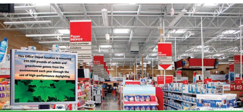
Example of green building design concepts being tested: daylight harvesting
